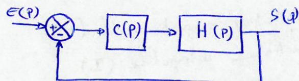
$$C(P) = k \frac{1 + T_i P}{T_i P} \quad \text{et} \quad H(P) = \frac{k_2}{1 + T_2 P}$$
