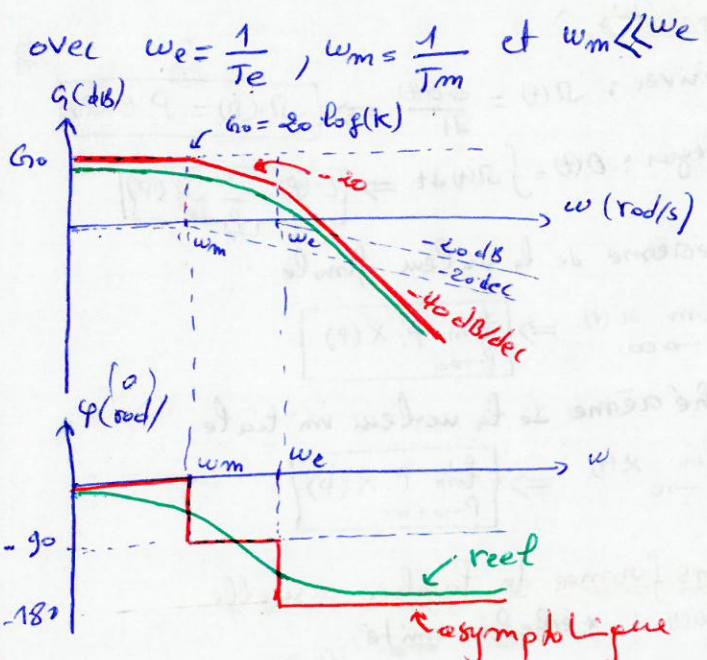
$$\left\{ |H| = \frac{K}{\sqrt{[1+(\frac{\omega}{\omega_e})^2][1+(\frac{\omega}{\omega_m})^2]}}$$
