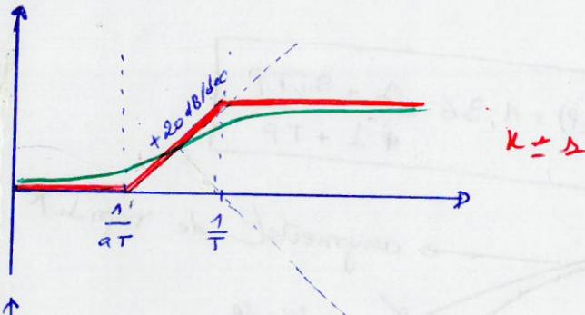
$$C(j\omega) = \frac{1 + \alpha T j \omega}{1 + T j \omega} = (1 + j \frac{\omega}{\omega_n})(\frac{1}{1 + j \frac{\omega}{\omega_n}})$$
