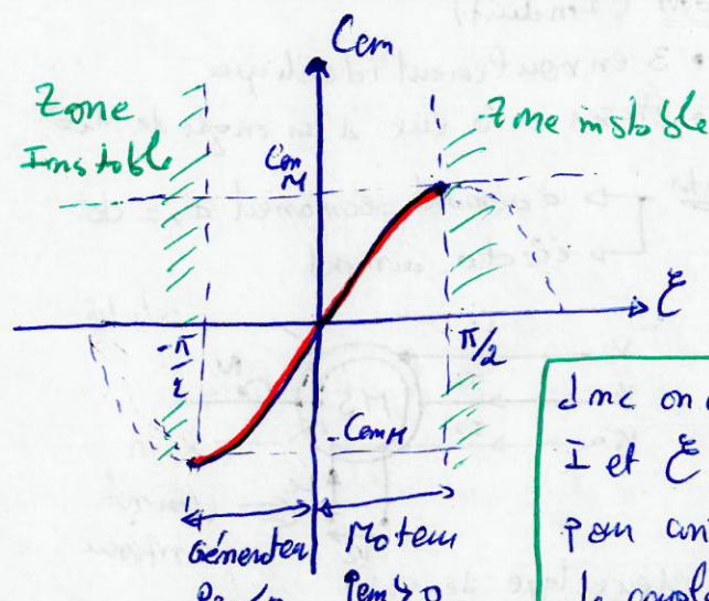
$$P_{\text{em}} \quad \boxed{\epsilon = \frac{\pi}{2}} \Rightarrow \boxed{C_{\text{em}} = C_{\text{em}}_{\text{max}} = 3 \cdot P \cdot \bar{\Phi} \cdot I}$$
